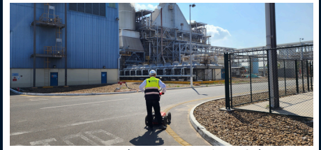
Concrete Scanning (Ground Penetrating Radar)- EGA
